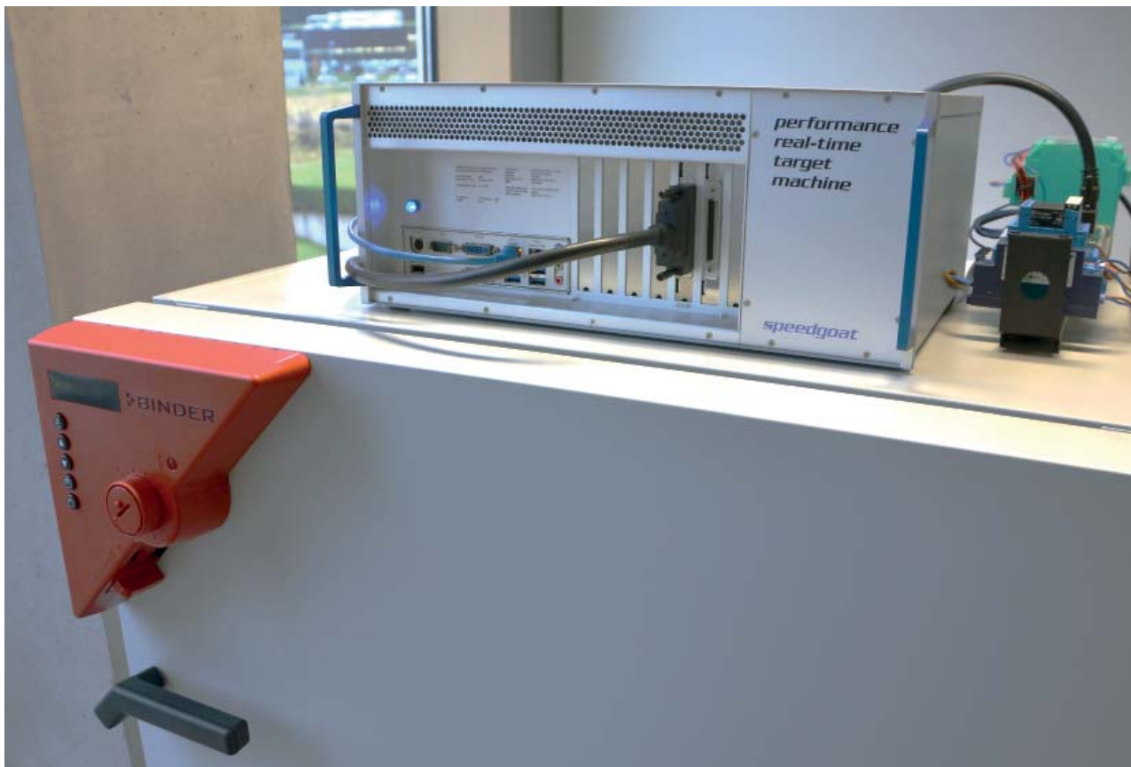
Running a new control algorithm on a Performance real-time target machine
