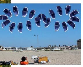
Small scale prototype built at UCSB with a tethered surf kite flying autonomous crosswind paths
