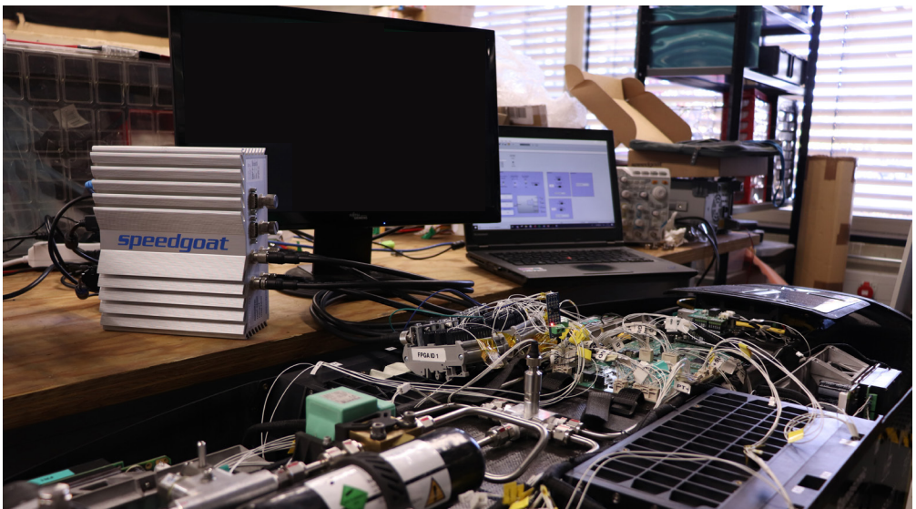
The TUM Hyperloop testing setup connecting the Baseline real-time target machine to the pod.
